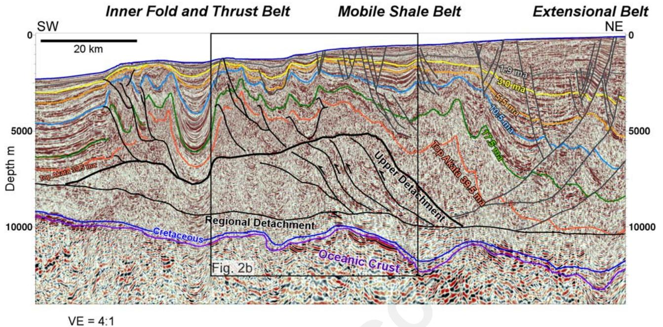
Figure 2A. The regional deep-tow, long-offset, PSDM seismic line located near the central delta, showing the shelf position into deep water and highlighting the Inner Fold and Thrust Belt (vertical exaggeration is 4:1). The seismic data is shown courtesy of ION Geophysical Inc.
