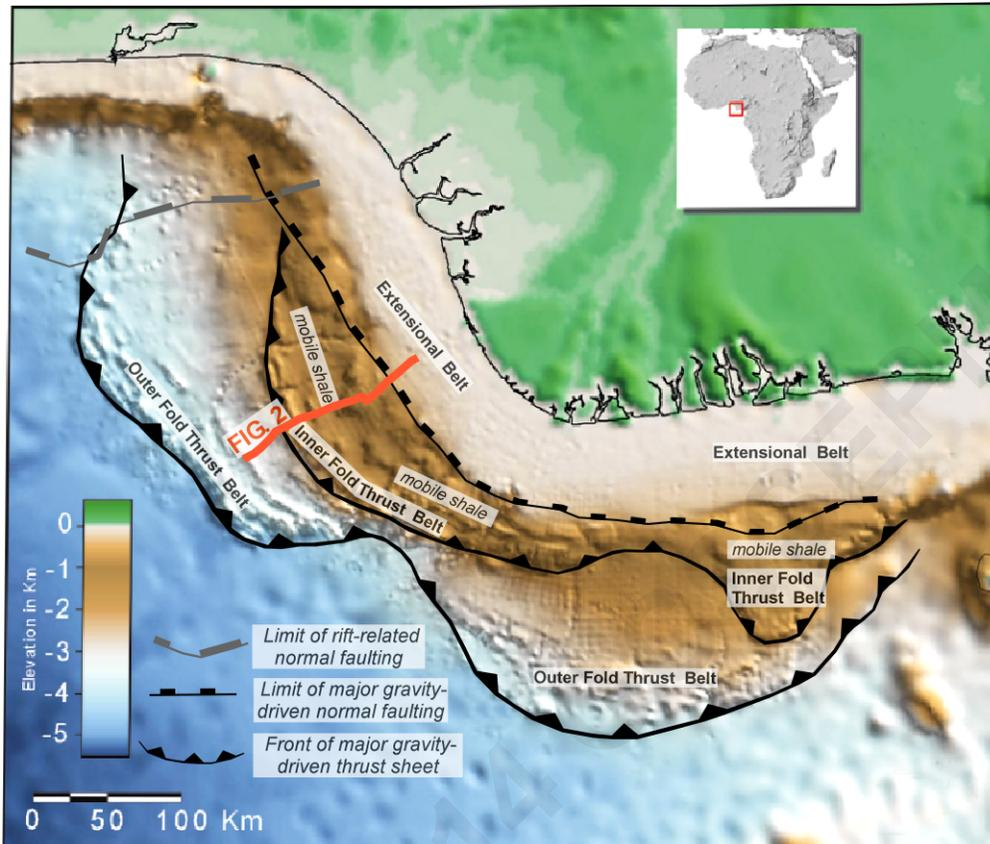
Figure 1. The Nigeria offshore base map with location of the key seismic line in bold red color. Major structural features of the delta are labeled shown over a bathymetric map from Corredor *et al.*, 2005.
