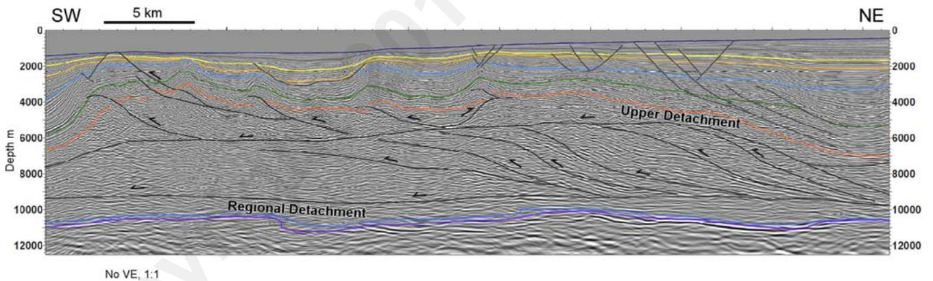
Figure 2B. Detail of Figure 2A shows the duplex feature consisting of an imbricated Akata shale section having an Upper (roof) Detachment and a (basal) Regional Detachment surface. The lower Miocene (17.5 Ma, green) to the Top Akata (39.5 Ma, orange) interval shows a variety of deep drilling targets, involved in folds and thrusts soling out onto the detachment surfaces (no vertical exaggeration). The seismic data is shown courtesy of ION Geophysical Inc.
