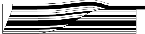
FIGURE 15. Models of curved-ramp fault-bend folding, with and without simple shear. The case of no shear (a) requires the progressive growth of a curved band a-a' at the base of the ramp, with bedding parallel to the fault, which is absent in end-member shear fault-bend folds such as (b) and (c). Also, slip goes to zero at the base of the ramp in the shear cases (b) and (c) with no bedding-parallel fault, whereas a basal fault of slip a-a' exists in the nonshear case (a). Therefore the effects of fault curvature and shear are distinguishable. Figures (b) and (c) also illustrate the effect of increasing shear zone thickness at constant displacement, which is to reduce the limb dips above the hanging-wall cutoff of the shear zone and to reduce the area of structural relief of the anticline. Notice that the input area of shortening decreases from (a) to (c).
